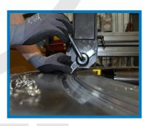
Set machine onto flange using setup fingers.
