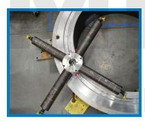
Extend feet into flange. Indicate, level and tighten leveling feet.
