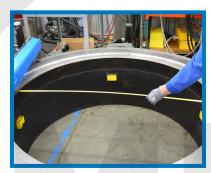
Lightly tighten leveling feet in the flange.
