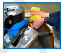
Assemble the ID chuck and install appropriate leg spacers.
