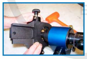
Select jaw set according to the ID diameter that the machine will chuck into.
